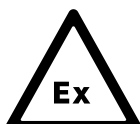
Fig. 0B - Warning sign for areas subject to the risk of explosion - Directive 99/92/EC
